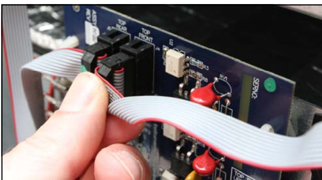
Figure 3: Unplug bezel from distribution board.
