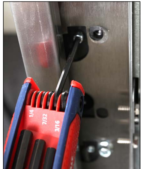
Figure 2: Remove 3/8 bolt and allen screw holding the bezel on each side.
