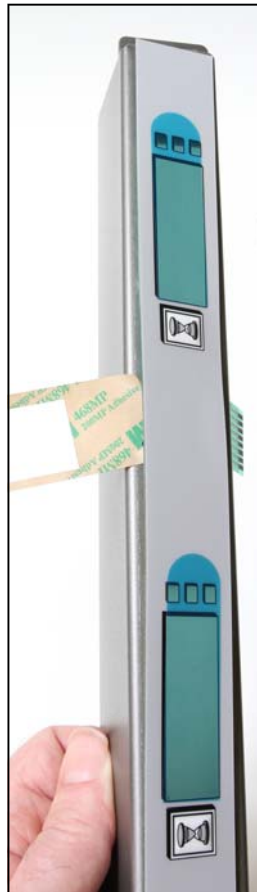
Figure 6: Scrape away the old adhesive and clean any oil residue on the metalwork.
