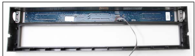
Figure 4: Four screws, two on each side, secure the metalwork to the bezel. Four screws, arrayed down the middle, secure the circuit board to the metalwork.
