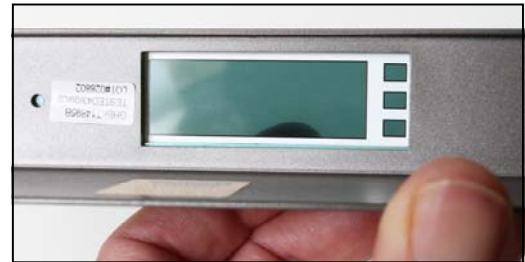
Figures 7-8: Remove a few inches of the adhesive backing (left) and ensure the windows on the membrane align with the rectangular openings in the metalwork (above).
