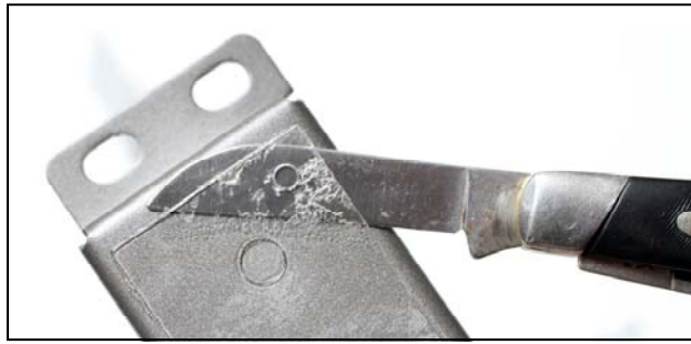
Figure 6: Scrape away the old adhesive and clean any oil residue on the metalwork.
